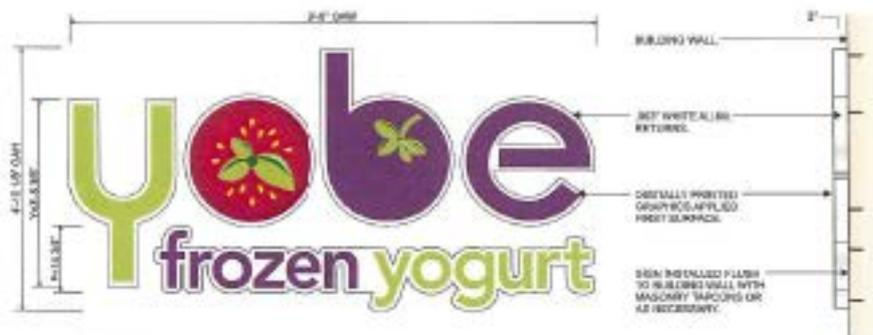
MANUFACTURE & INSTALL ONE (1) SET OF CUSTOM NON-ILLUMINATED CORNER LETTERS, 1/2" ALUMINUM FRAMES DIGITALLY PRINTED 3M U-100C WHITE VINYL, & 3M 8330 (LAMINATE APPLIED) FIRST SURFACE, 3" DEEP ALUMINUM RETURNS PAINTED PMS WHITE 90 ALUMINUM ANGLE SUPPORTS, ENDS TO BE WELDED TO RETURN LETTERS TO BE FLUSH MOUNTED TO EXISTING BUILDING WALL.
