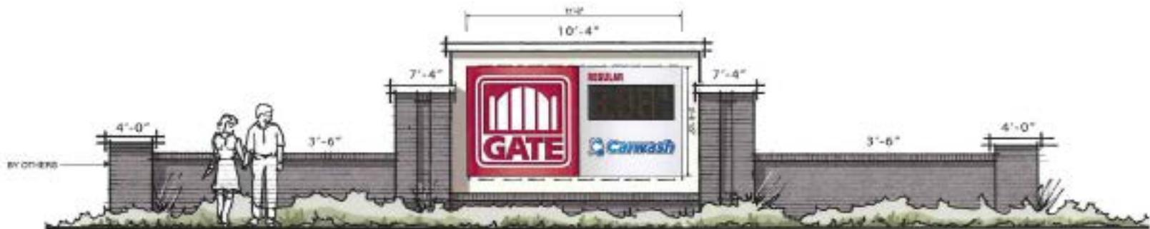
MANUFACTURE & INSTALL 1 CABINET FOR 1 MONUMENT INTERNALLY ILLUMINATED 5'6" WALL SIGN. "GATE" TO BE 3/16" THICK FINNED WHITE ACRYLIC FACE W/ 3M 3636-33, RED TRANSLUCENT VINYL GRAPHICS APPLIED FIRST SURFACE. CABINET TO BE INTERNALLY ILLUMINATED W/ WHITE LEDs. GAS PRICER ALUMINUM FACE TO BE PAINTED AKZO NOBEL BRN 10 SILVER.
