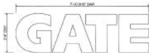
12 Front Elevation & Sign Detail - Standard Channel Letters
