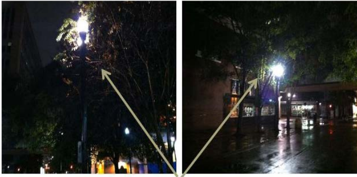
A large number of installed lighting (particularly in the Hemming plaza park area) were either obstructed, or fully concealed by existing vegetation. As a result, numerous concealment areas, and dark locations were created.
