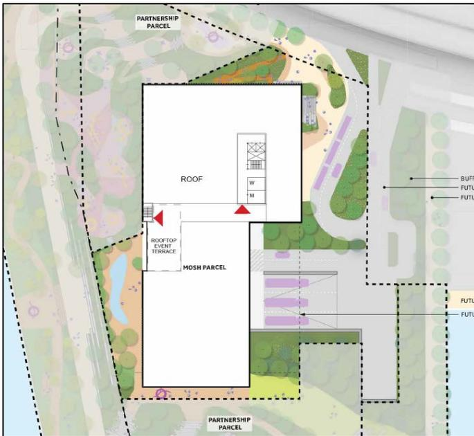
As currently designed, the proposed roof plan is mostly flat, activated with a rooftop event terrace and circulation to the event terrace. The terrace itself is isolated to a small area of the roof along the eastern edge of the building.
