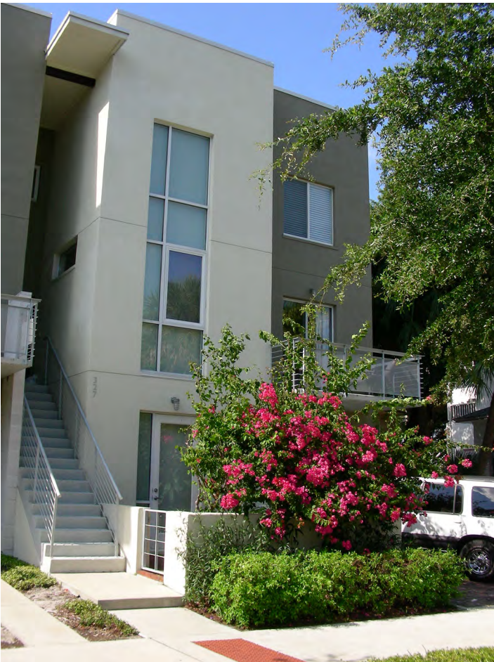
Do - An elevated floor level creates additional privacy for ground floor residential units. Stoops and porches create outdoor open space for ground level units.
